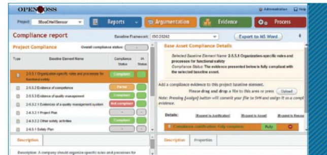
FIGURE 6. The compliance management panel summarizes which ISO 26262 requirements our project has fulfilled and to what extent we've covered all the requirements.
