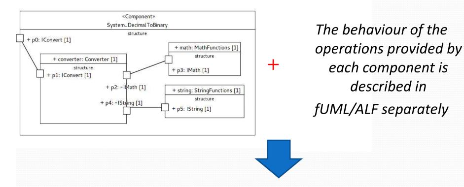
An fUML/ALF executable model of the whole SW architecture
