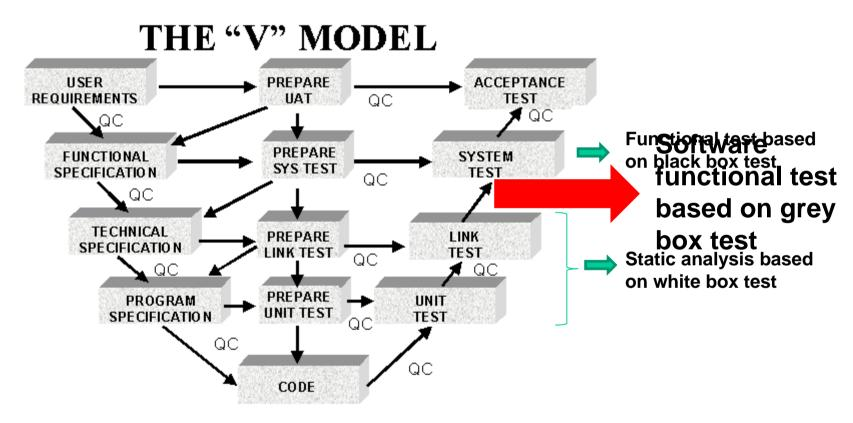
The aim is to test only the software functionalities on real target
